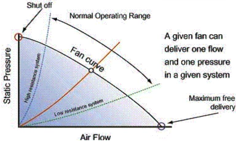
This non-linear expression of airflow versus static pressure can be stated as:
